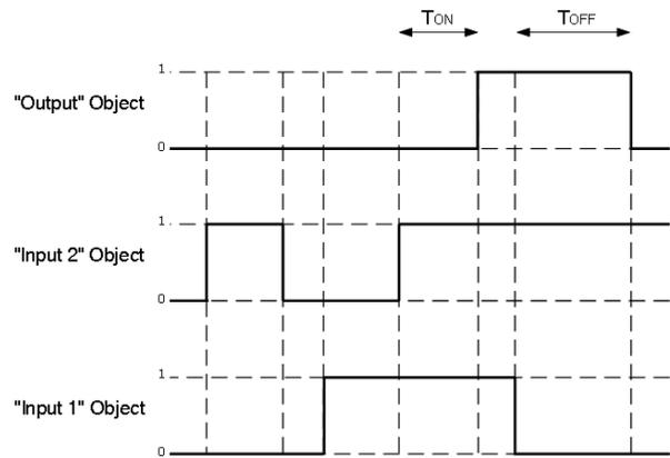
Fig1. Logic Gate with delays
