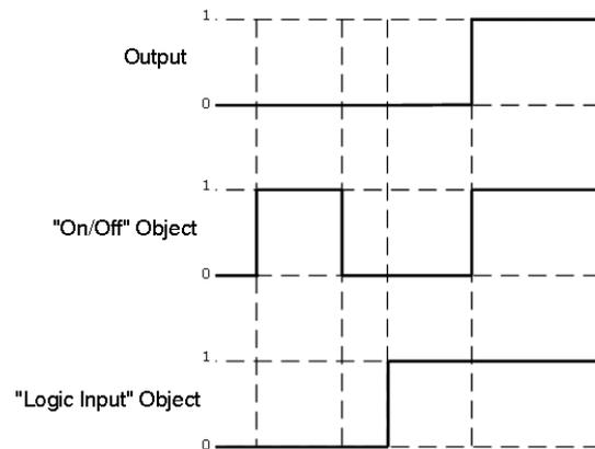
Fig8. AND Logic Function
