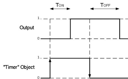
Fig4. ON/OFF Delays
