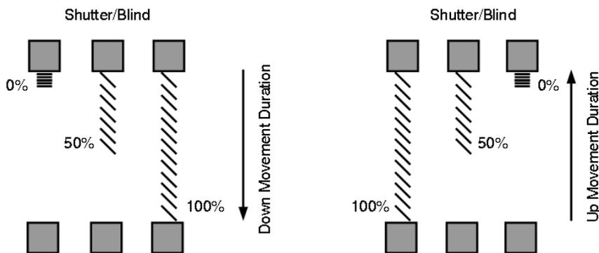
**Fig19. Shutter/Blind Movement Duration**
