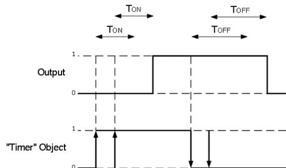
Fig5. ON/OFF Delays Retriggerable
