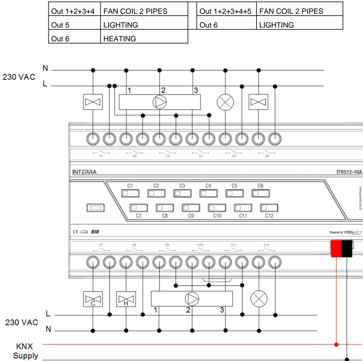
**Fig22. Connection Diagram Example Configuration 2**
