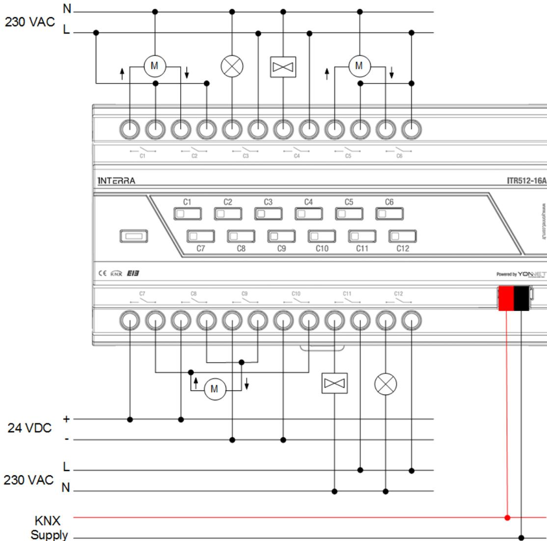
**Fig23. Connection Diagram Example Configuration 3**
