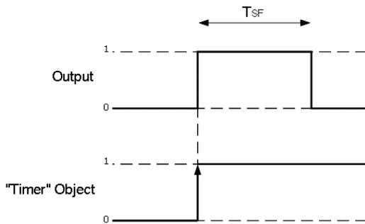
Fig2. Staircase Function
