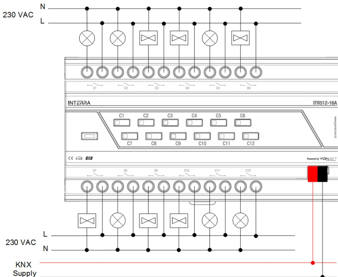
Fig21. Connection Diagram Example Configuration 1
